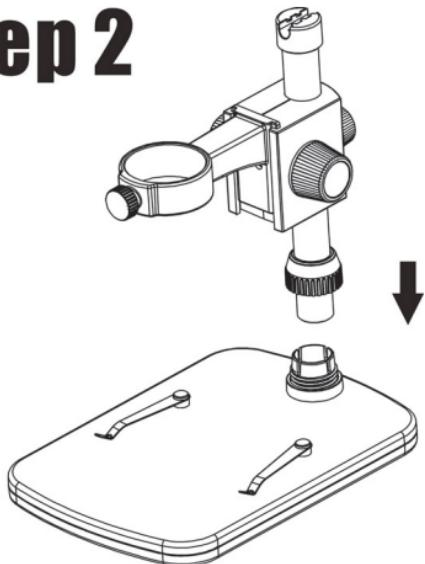
**Put the metal pole into the female part of the stage.**
