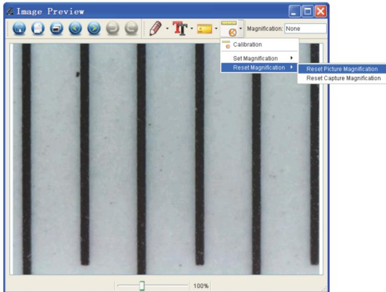
2). Change the magnification rate and capture several pictures, click on the picture to enter into measurement
